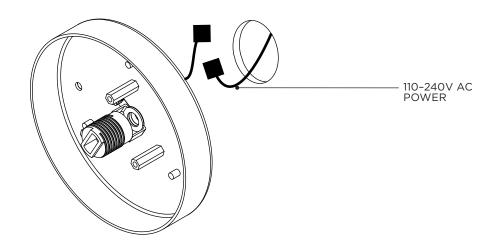
With the electrical connection made, push back wiring into wall cavity and screw fix WALL MOUNT MODULE to the wall. Ensure the wall fixing fasteners are secured to an adequate load bearing substrate.
