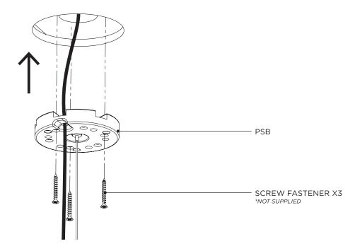
**9** Raise the PENDANT, feeding excess cable through the CABLE GLIDERS. Set into position by gently lowering the PENDANT.
