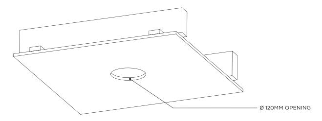
Installer to provide adequate load-bearing substrate, utilising ceiling joists where additional support is required. The mounting face of the substrate must be set back 20mm from the ceiling facade. For accurate placement of Cable Exits in the Substrate, use the PSB as a guide or refer to the provided template at the end of this document.
