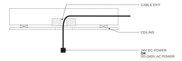
From the pendant, feed the SUSPENSION WIRE through the central hole in the ESCUTCHEON and POWER CABLE through the CORD GRIP as shown.
