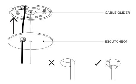
With the ESCUTCHEON in place, ensure the CORD GRIP is adequately tightened on to the POWER CABLE and make any necessary final adjustments to the PENDANT.
