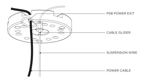
Connect the POWER CABLE from the PENDANT to the 24V DC power supply OR the 110-240V AC cable. Refer to supplied WIRING DIAGRAM →
