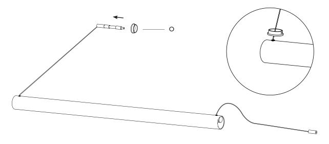
13. Slide the medium tube (R) onto the lighting assembly (S) until it is placed in the middle. Then, slide the larger tube (T) onto the medium tube (R) until it is placed in the middle.
