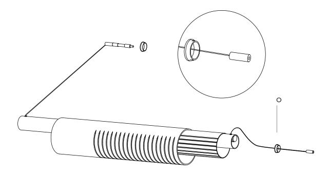
15. Thread the metal endcap (N) back onto the threaded rod in the tube.
