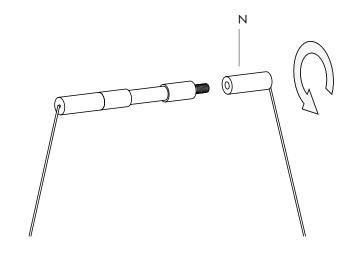
11. Unthread both endcaps (P) from the hanging mechanism, take off the top cap (Q) and put those three elements (P,O,Q) aside for later.
