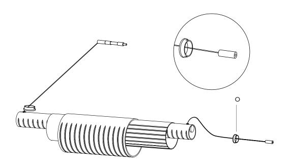
15. Thread the metal endcap (N) back onto the threaded rod in the tube.
