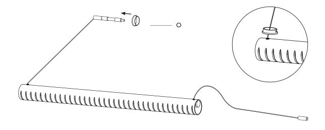
13. Slide the medium tube (R) onto the lighting assembly (S) until it is placed in the middle. Then, slide the larger tube (T) onto the medium tube (R) until it is placed in the middle.
