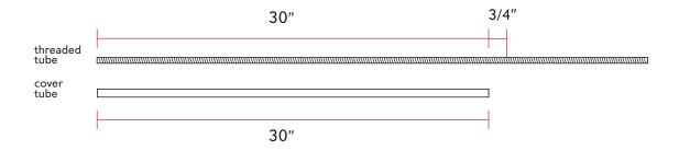
4. Hold down the all thread with a hand or a clamp, use a hacksaw or electrical tool to cut the all thread tube. Recommended to clean all thread tube after cutting to remove any metal chippings.
