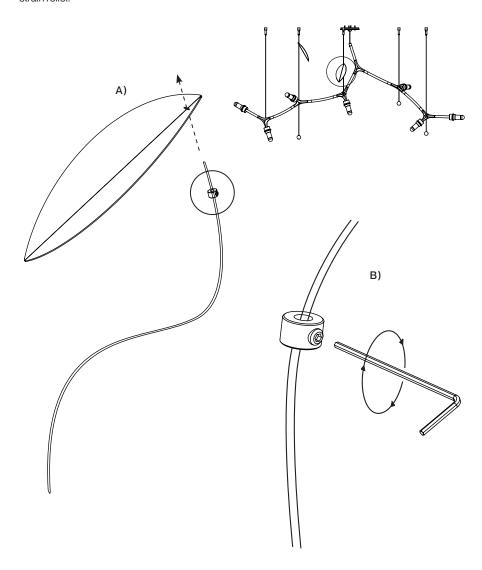
**08.**Adjust chandelier height as needed using the cable griplocks.
