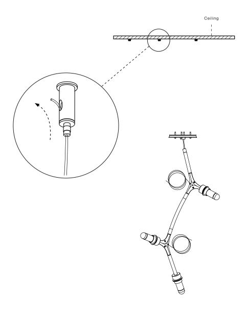
For all leaves above fixtures: Pass the stainless cable through the small silver strain relief. Place it to the lowest height above fixture suggested on the cover image and tight the set screw with the appropriate allen key. Then, pass the cable through the appropriate leaf and let the leaf hang on the strain relief.
