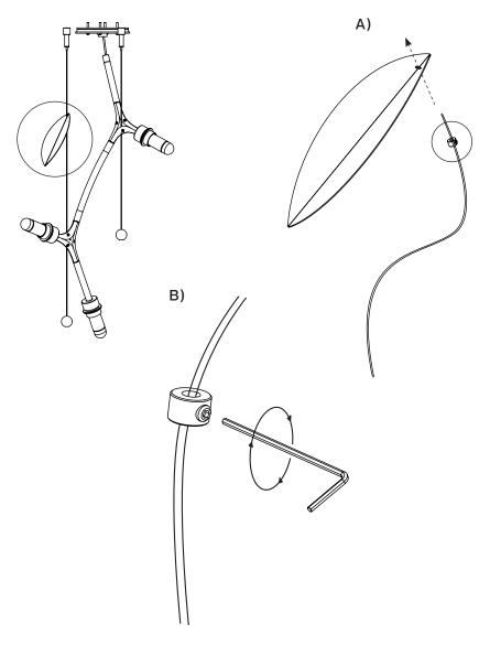
Adjust chandelier height as needed using the cable griplocks.
