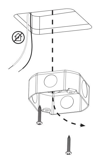
Using wire terminals, connect the LED driver to the main power source. Secure the LED driver in remote location by also making sure to keep access to the output wires. Make sure to keep the driver inside a 100 ft distance of the fixture. Refer to the driver documentation for more informations.
