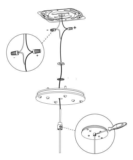
Using provided screws, install the fixture to the universal cross bar.
