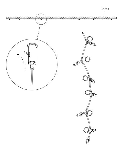
For all leaves above fixtures: Pass the stainless cable through the small silver strain relief. Place it to the lowest height above fixture suggested on the cover image and tight the set screw with the appropriate allen key. Then, pass the cable through the appropriate leaf and let the leaf hang on the strain relief.
