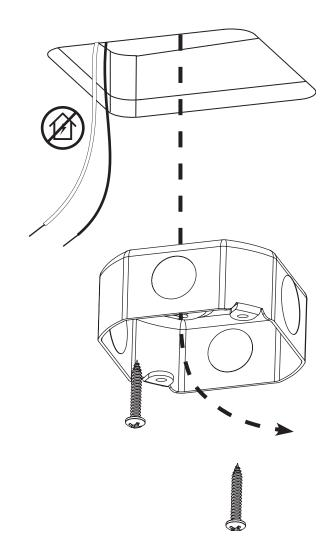
Using wire terminals, connect the LED driver to the main power source. Secure the LED driver in remote location by also making sure to keep access to the output wires. Install the driver within 100ft of the fixture. Refer to the driver documentation for more informations.
