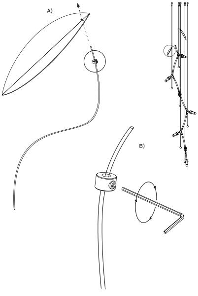
Adjust chandelier height as needed using the cable griplocks.
