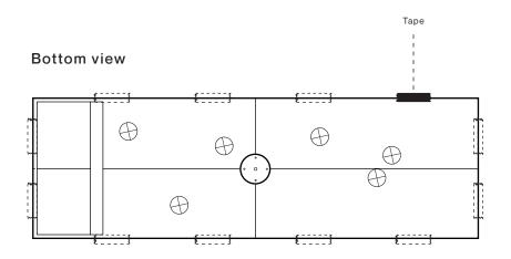
Install all female monopoints at the cross indicated on the template. Note: Use achors rated for a minimum of 25lbs.
