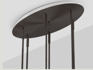
CIRCULAR FIXED SWIVEL CANOPY CAN.VC.CIR.SW.X-XXX Ø600 X 37MM / 23.6" X 1.5" DRIVER HOUSED IN CANOPY
