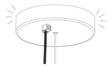
Conduct a final visual assessment of both the canopy and fixture to 12 ensure all parts have been properly fitted and secured. Once satisfied that everything is in working order remove all remaining protective material which will now complete the installation process.
