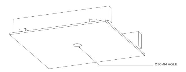
Installer to provide adequate load-bearing substrate, utilising ceiling joist where additional support is required.
