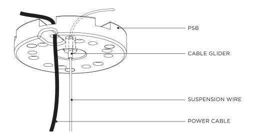
Connect the POWER CABLE from the PENDANT to the 24V DC power supply OR the 120-240V AC cable. Refer to supplied WIRING DIAGRAM →
