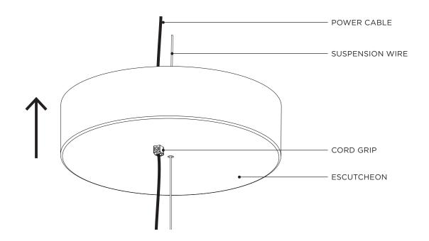
Feed the SUSPENSION WIRE through the CABLE GLIDER followed by the POWER CABLE through the PSB POWER EXIT.
