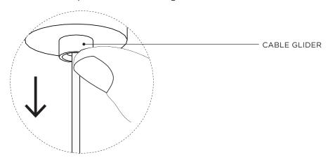
Carefully raise ESCUTCHEON to the ceiling until the Magnets engage. 10 Ensure no contact between ESCUTCHEON and CABLE GLIDER, as this may release the suspension wire.
