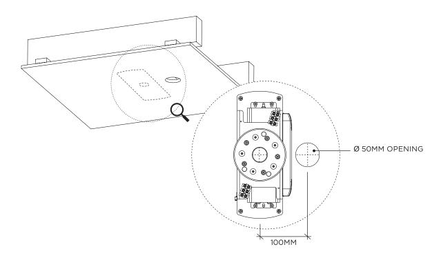
Installer to provide adequate load-bearing substrate utilising ceiling joist where additional support is required.
