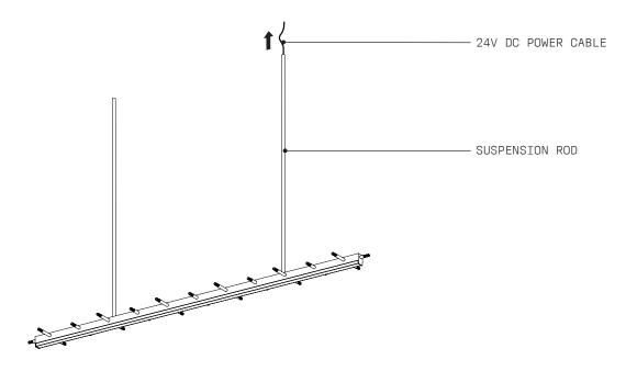
Once the fixture is suspended and secure, unwrap the quartz slices and begin to place them on to the ALLTHREAD, starting with the shorter COUPLERS. Fasten the Quartz in place using the provided FINIALS, ensure to put on the opposite slices to maintain the balance.
