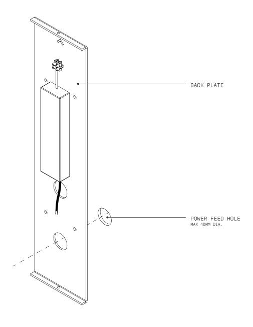
Pull POWER CABLE through POWER FEED HOLE in BACK PLATE, and fix BACK PLATE to the wall.
