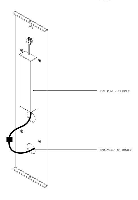
5 Feed ELECTRICAL CABLE through CORD GRIP in brass ESCUTCHEON. Connect ELECTRICAL CABLE to 12V POWER SUPPLY.
