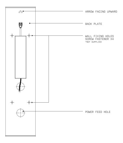
Remove the BACK PLATE and cut the POWER FEED HOLE.
