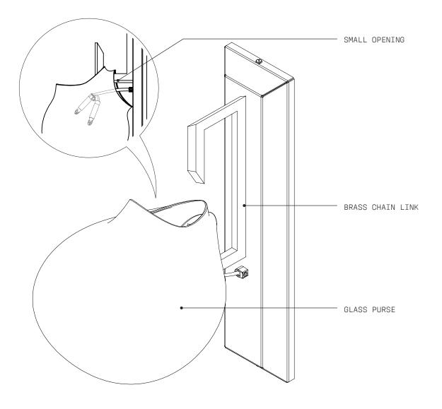
Switch the power ON and conduct a final visual assessment to ensure all parts have been properly fitted and secured. Ensure G4 LAMPS are not hanging too low, as this will create hot-spots on the GLASS PURSE.
