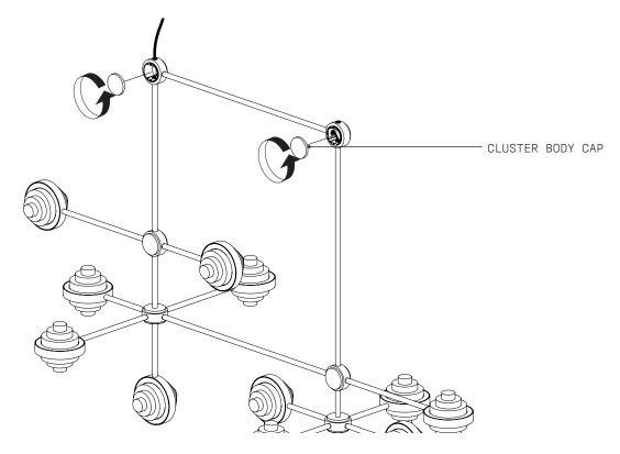
$3\,$   $\,$  Loosen the 2x upper most GRUB SCREWS to release the HEX NIPPLE.
