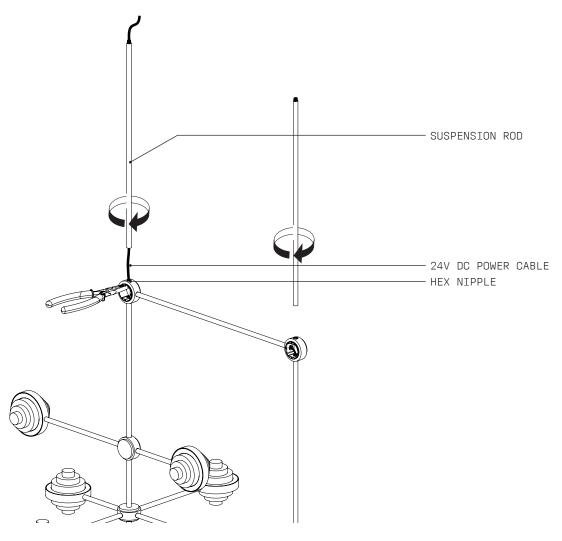
5 Tighten the 2x upper most GRUB SCREWS.
