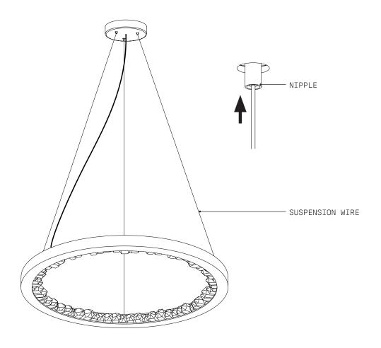
Adjust the level of the fixture using the adjustable CABLE GLIDERS. The lengths of the SUSPENSION WIRES can be adjusted to be lower by taking the weight off the suspension wire, and pushing on the spring loaded NIPPLE on the CABLE GLIDER
