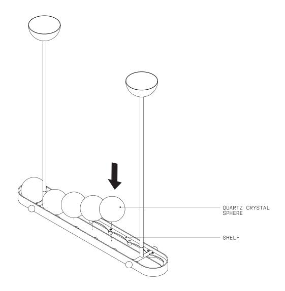
8 Conduct a final visual assessment of the fixture to ensure all parts have been properly fitted and secured. Once satisfied that everything is in working order, remove all remaining protective material which will now complete the installation process.
