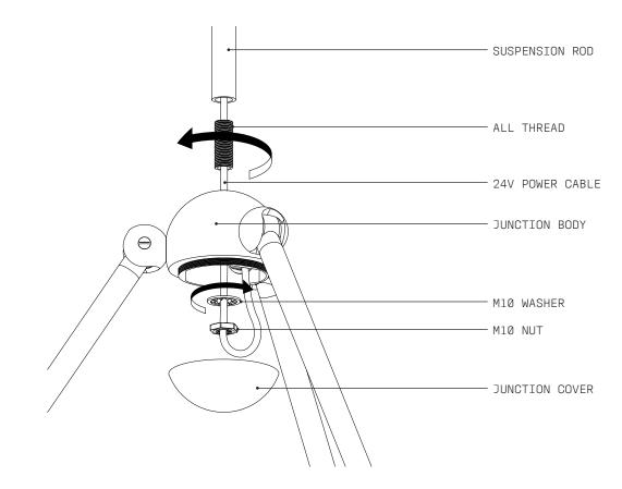
Ensure that the PENDANT is the right way up as per diagram. Feed the 24V DC POWER CABLE
