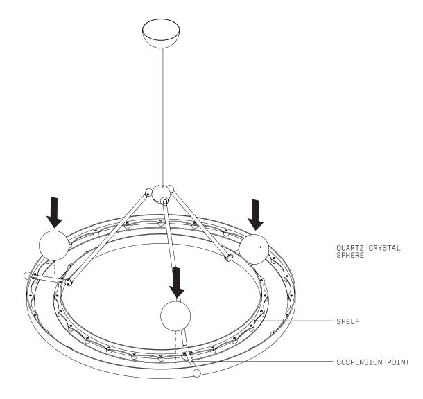
8 Conduct a final visual assessment of the fixture to ensure all parts have been properly fitted and secured. Once satisfied that everything is in working order, remove all remaining protective material which will now complete the installation process.
