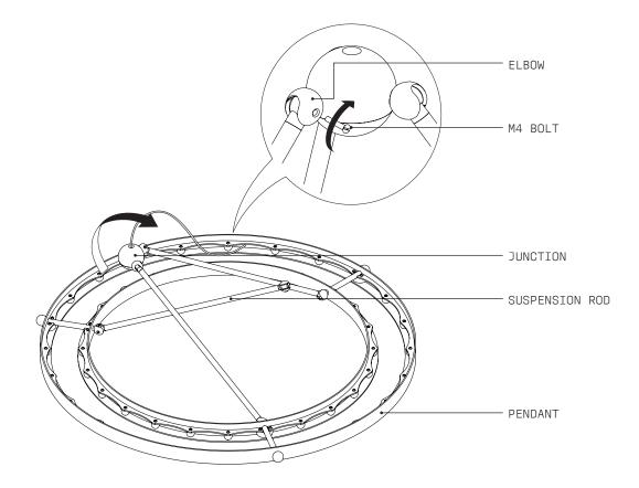
Twist and remove JUNCTION COVER and thread SUSPENSION ROD on to JUNCTION BODY using
