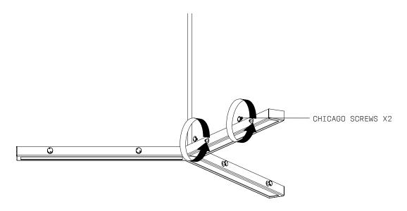
5 Carefully place 1x BUCKY VITRINE GLASS over the 2x SUPPORTS and firmly tighten the 2x CHICAGO SCREWS to safely secure the glass.
