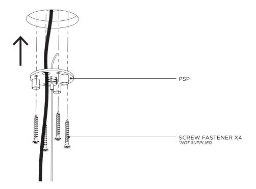
**9** Raise the PENDANT, feeding excess cable through the CABLE GLIDERS. Set into position by gently lowering the PENDANT.
