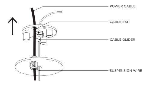
Connect the 24V DC or 110-240V AC POWER to the POWER CABLE. Refer to supplied WIRING DIAGRAM →
