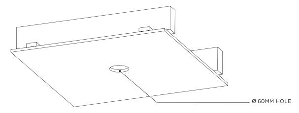
Installer to provide adequate load-bearing substrate, utilising ceiling joists where additional support is required. The mounting face of the substrate must be set back 15mm from the ceiling facade. For accurate placement, refer to the DRILLING TEMPLATE on the last page of this document.
