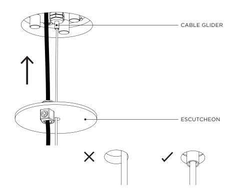
With the ESCUTCHEON in place, ensure the CORD GRIP is adequately tightened on to the POWER CABLE and make any necessary final adjustments to the PENDANT.
