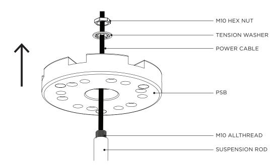
Connect the 24V DC or 110-240V AC POWER to the POWER CABLE. Refer to supplied WIRING DIAGRAM→
