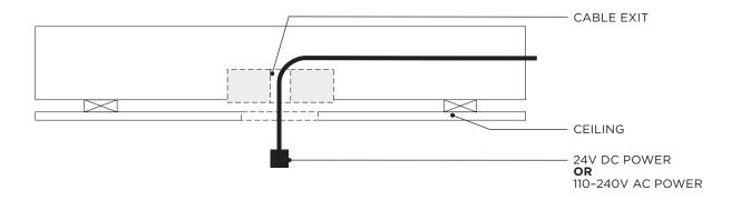
From the pendant, feed the POWER CABLE & SUSPENSION ROD through the central hole in the ESCUTCHEON as shown ensuring not to scratch the suspension ROD.
