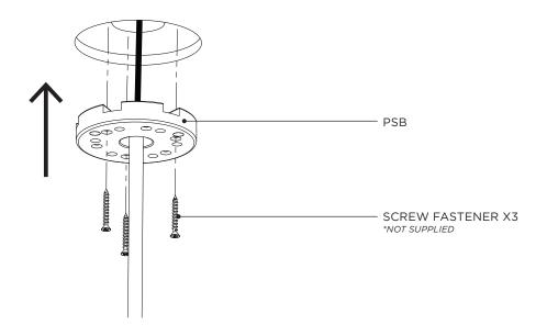
Carefully raise ESCUTCHEON to the ceiling until the Magnets engage. Ensure not to damage the SUSPENSION ROD as the ESCUTCHEON is being raised.
