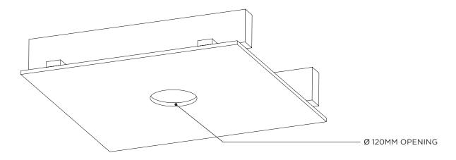
Installer to provide adequate load-bearing substrate, utilising ceiling joists where additional support is required. The mounting face of the substrate must be set back 20mm from the ceiling facade. For accurate placement of Cable Exits in the Substrate, use the PSB as a guide or refer to the provided template at the end of this document.
