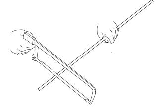
3. Now that the cover tube is cut to 31.5", measure the all thread tube to be 32" long. And place a mark, with a marker or tape.
