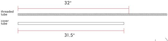
4. Hold down the all thread with a hand or a clamp, use a hacksaw or electrical tool to cut the all thread tube. Recommended to clean all thread tube after cutting to remove any metal chippings.
