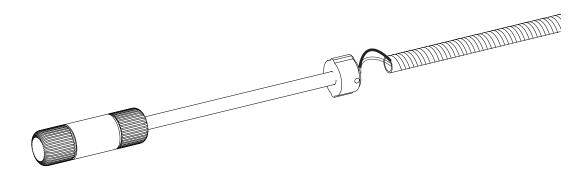
3. Slide the cover tube onto the threaded tube, and stackup the two threaded nuts + canopy with the order and orientation shown below:
