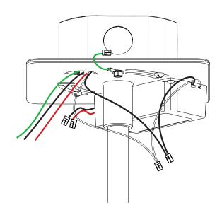
7. Make the electrical connection between the J-box and fixture.
