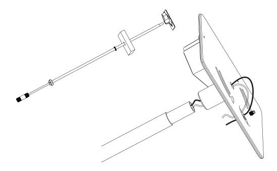
5. Make the connection between the LED stem and the driver by connecting with the provided wagos
