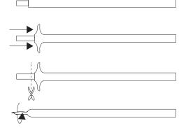
4. Set griplock to desired drop and tighten the safety nut.
