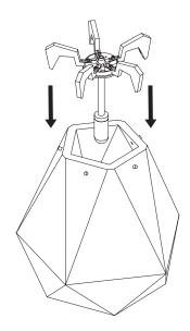
STEP 4 Push the spider legs inwards so that the holes align with the nipples protruding from the glass and tighten the screws down. Screw the lobed locknut over the entire assembly
